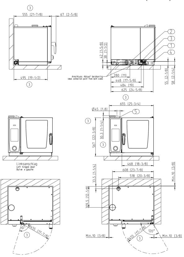
1. Common water supply (cold water) "Single" water connection as shipped 2. Drain 2" OD 3. Electrical connection wire entrance 4. Chassis Ground connection 5. Steam Vent pipe 2 3/8" / 60mm Minimum Clearance 2" / 50 mm Left side clearance 20" recommended for servicing of unit without the ability to move unit while connected. Measurements in mm (inch)
