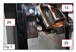
2. Release the bag grip while holding the 2 side supports and unscrew the 2 top bag grip fixing screws (24). (fig. G)
