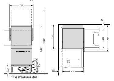
① Drain hose ② Supply hose ③ Connection cable ④ Liquid detergent  $^{a)}$  ⑤ Rinse aid  $^{a)}$  depending on the device chemical dispensers are not included
