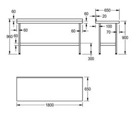
Midi wall tables will align with the Midi range of catering sinks. Midi wall tables are manufactured from 1.2 thick austenitic grade stainless steel polished to a satin finish. Stainless steel underframes complete with shelf are supplied with each table, in a flat pack form with easy to read assembly instructions. Each leg is fitted with an adjustable foot (-20, +10mm) with a working height of 900mm.
