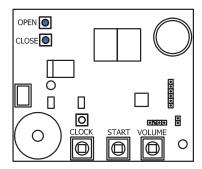
6.2.10 To adjust the clock: Press the CLOCK (left) button. The display will show the hour (24hr clock). Hold for 5 seconds and until the current hour is displayed. You will hear a ticking sound as the display advances.
