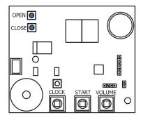
6.2.10 To adjust the clock: Press the CLOCK (left) button. The display will show the hour (24hr clock). Hold for 5 seconds and until the current hour is displayed. You will hear a ticking sound as the display advances.
