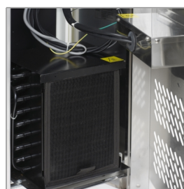
Easy access to clean dust filter
