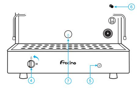
4) To ignite the burner turn the main gas regulator/isolation valve on.
