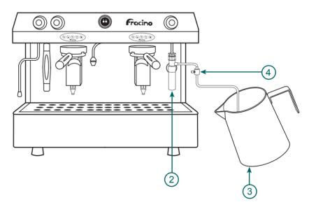
2) Carefully attach the the Idea Rapido frother in place of the removed steam tube taking care not to overtighten.
