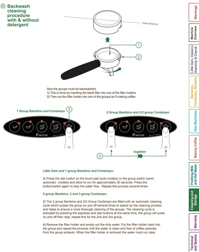
On a daily basis the back washing process should be done using Fracino Liquid Quartz detergent to reduce the build up of coffee in the groups and solenoid valves. This can be purchased through your dealer or from Fracino direct (part no. DET/LIQUID) Put half a cap of detergent into the blank insert and follow backwash procedure.
