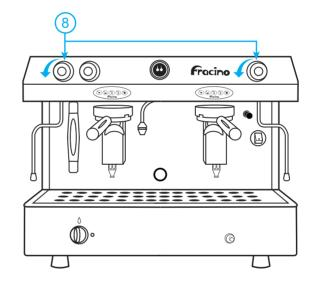
8) Once steam starts to pass through the steam tube (approximately 15 minutes using electricity or 30 minutes using gas from switching machine on) close the valve. The pressure will be then build up to 1.0 - 1.2 BAR.
