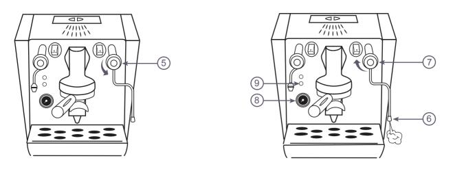
5) Open the steam valve by turning the black handle anti-clockwise.
