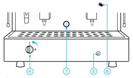
4) To ignite the burner turn the main gas regulator/isolation valve on.
