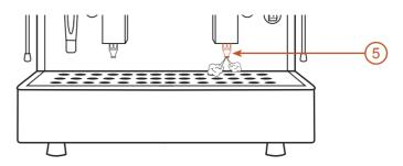
5) Press the button to start the coffee flow as shown below. Once the coffee flow stops any excess pressure that is left in the filter holder is discharged through the exhaust valve below the group. Remove the filter holder from the group, empty used coffee grounds into drawer or receptacle and place empty filter holder back in the group to keep it warm.
