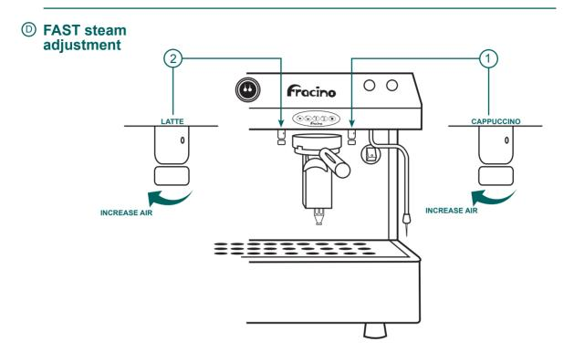
The volume and texture of the milk foam can be adjusted for the cappuccino and latte by adjusting the cappuccino and latte adjusting valves.
