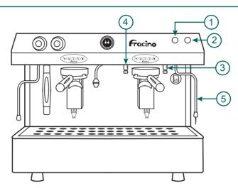
1) Cappuccino/Latte selector switch: Selects between cappuccino and latte milk. 2) Start cycle switch: Starts the milk frothing cycle.
