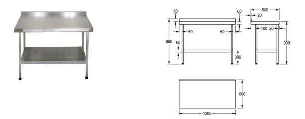
Mini wall tables will align with the Mini range of catering sinks. Mini wall tables are manufactured from 1.2 thick austenitic grade stainless steel polished to a satin finish. Stainless steel underframes complete with shelf are supplied with each table, in a flat pack form with easy to read assembly instructions. Each leg is fitted with an adjustable foot (-20, +10mm) with a working height of 900mm.
