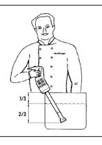
Always make sure that the bell is sufficiently immersed to avoid splashing and that the air vents of the motor unit does not come into contact with any liquid.
