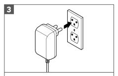
Plug the Charger Adapter into an earthed electrical outlet.
