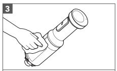
Wipe the Motor Body with a damp cloth. Mild dish soap may be used, but do not use abrasive cleansers.
