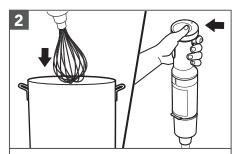
Insert the Cordless Hand Blender into the mixture. Press the Variable Speed Controller and Palm Switch at the same time to start.
