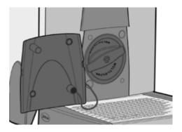
3. Grip Cartridge and rotate a quarter-turn to the left and pull forward. CAUTION: A small amount of water will drain from the head.
