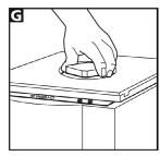
WARNING: When replacing the front of panel, ensure that wires do not get trapped between tap and front panel.
