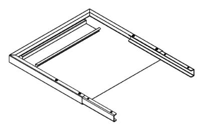
6.6 Slide fitted splashback onto main body as shown. **Ensure bowl splashback sits behind main body splashback.** Once the splashback is placed into position and holes align, fit screws.
