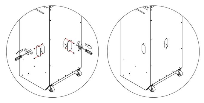
6.8 If needed, remove cover plates to run water and waste services, as appropriate.
