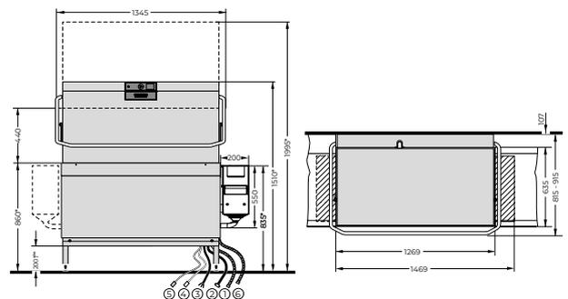
Maximum table profile height with AMXXL and AUPL in corner installation: 40 mm.
