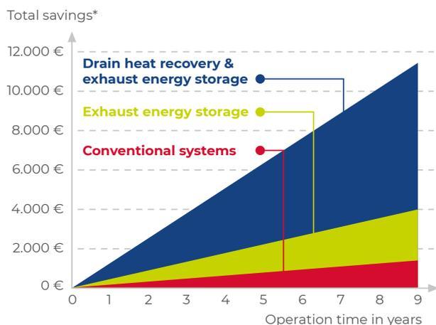
\* Calculation basis: AMXT with 100 cycles/day, 312 days/year, energy costs: 0.23 €/£0.19/kWh, volume of rinse water: 2.0 l/rack
