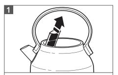
**To access Filter:** Open the Lid; the Filter is located behind spout inside Electric Kettle. Grasp the top of the Filter to remove.
