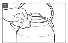
The exterior of the Electric Kettle may be cleaned with a damp cloth. Dry and polish the Electric Kettle with a soft cloth. Abrasives and scouring agents of any kind are not recommended.
