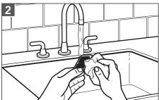
Clean under hot water with a soft brush or cloth to remove deposits, and replace Filter by sliding the Filter into the slot behind the spout.
