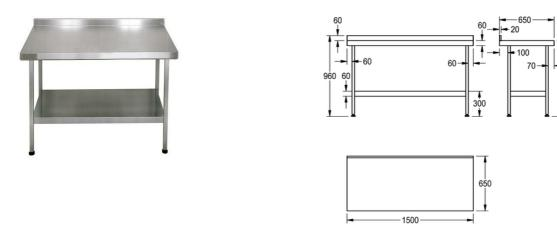
Midi wall tables will align with the Midi range of catering sinks. Midi wall tables are manufactured from 1.2 thick austenitic grade stainless steel polished to a satin finish. Stainless steel underframes complete with shelf are supplied with each table, in a flat pack form with easy to read assembly instructions. Each leg is fitted with an adjustable foot (-20, +10mm) with a working height of 900mm.
