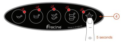
**4)** Press the star button on the left hand touch pad and hold for 5 seconds until the lights above the symbols start to flash. The machine is now in program mode.
