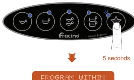
4) Press and hold the star button on the left hand keypad for approximately 5 seconds until the LED on the star button flashes on and off. The display will read "PROGRAMME WITHIN 30 SECONDS".
