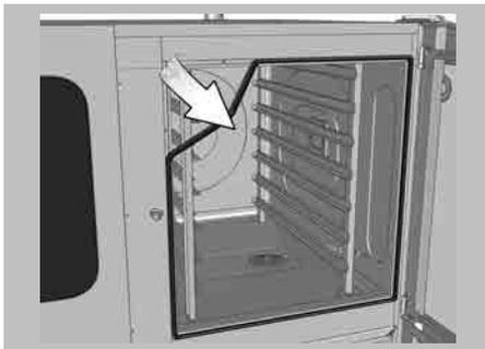
Pull out the hygienic plug-in gasket around the appliance door opening. Start from the corners.
