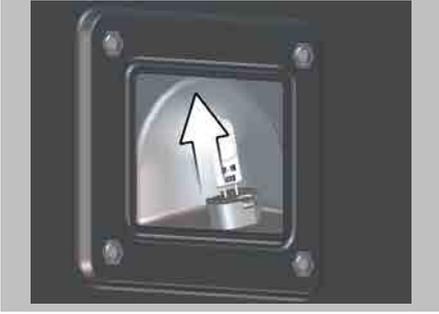
3. Reach into the reflector housing through the opening on the cooking compartment wall and pull out the halogen lamp upwards in a straight line.
