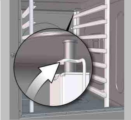
Check to make sure that the retainers on the rear top corners are engaging the racks properly so that the latter are correctly secured.
