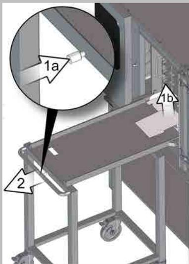
Release the transport trolley's engaging mechanism from the cooking compartment opening and move the trolley away.
