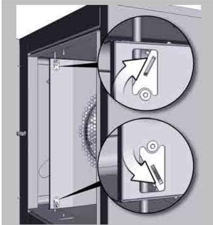
Release the upper and lower latches with the tool.
