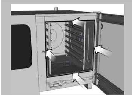
Once all four corners are in place, meticulously press the hygienic plug-in gasket into the rest of the guide. Make sure that the hygienic plug-in gasket is resting solidly against the guide and that there are no bends or kinks in it.
