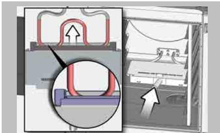
Grab the smoker box containing the bisquettes from the handle and slide it all the way onto the smoker heater inside the cooking compartment. Make sure that the heating element goes into the smoker box opening meant for the smoker heater.
