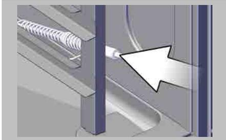
Slide the core temperature probe into the spiral holder on the right-hand side rack.
