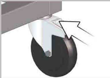
Release the transport trolley's parking brakes.
