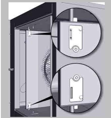
Check to make sure that the upper and lower latches are engaged.
