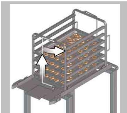
Lift the tray guard bar at the back of the mobile shelf rack and swing it to the right side.
