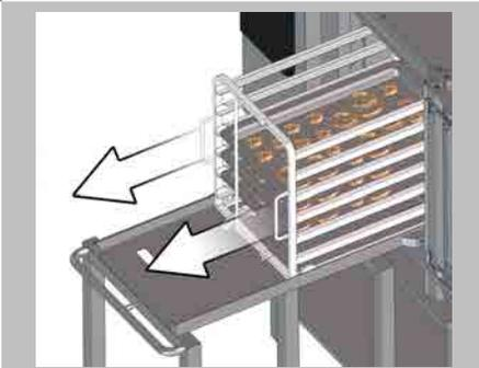
Pull the mobile shelf rack out from the cooking compartment and onto the transport trolley.
