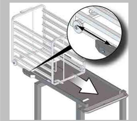
Slide the mobile shelf rack onto the transport trolley from behind. Make sure that the wheel axles go under the transport trolley’s hem.
