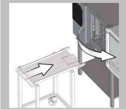
Open the appliance door and move the trolley in front of the combi steamer.
