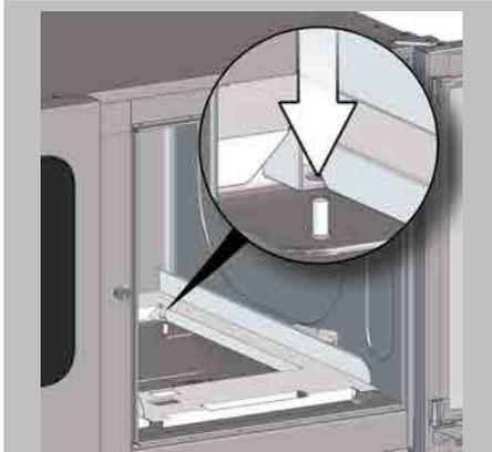
Secure the roll-in frame inside the cooking compartment by guiding the holes on the roll-in frame's foot angle brackets onto the pins on the bottom of the cooking compartment.
