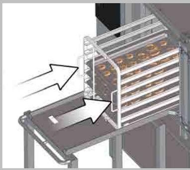
Slide the mobile shelf rack away from the transport trolley and into the cooking compartment.
