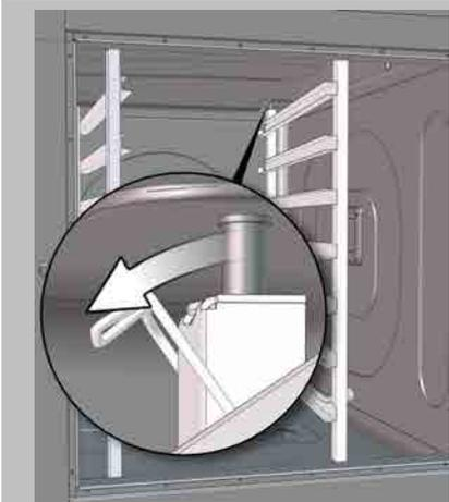
Release the retainer on the rear top corner that is holding the rack in place.
