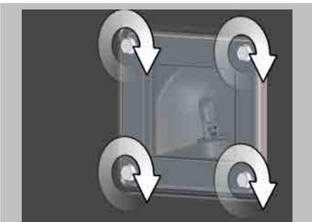
1. Follow the same steps used to remove the halogen lamp, but in opposite order. Once you are done, remove all objects from the cooking compartment. Then rinse or wipe the cooking compartment clean.
