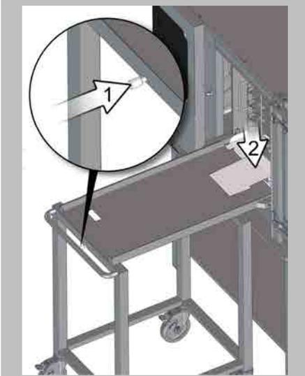
Secure the transport trolley on the combi steamer.
