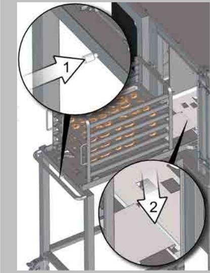
Secure the transport trolley on the combi steamer.
