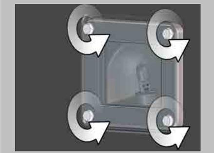
1. Remove the four oven light hex screws using the socket wrench. Due to its design, the assembly consisting of the screws, bezel, glass pane, seal, and bracket will remain together when the screws are unscrewed.
