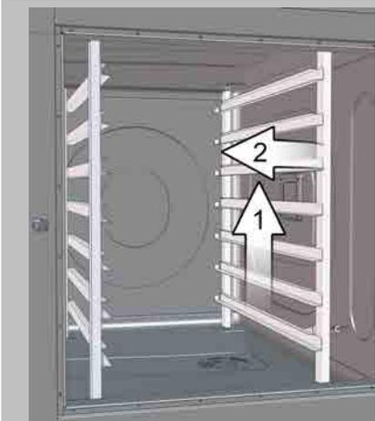
Lift (1) the rack and swing it (2) towards the inside of the cooking compartment.
