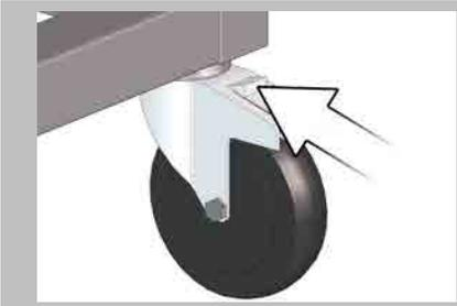
Release the transport trolley's parking brakes and move the trolley in front of the combi steamer.
