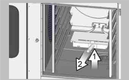
Insert the handle into the smoker box and pull the box out from the smoker heater.
