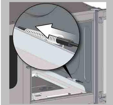
Slide the core temperature probe into the spiral holder on the right side of the roll-in frame.
