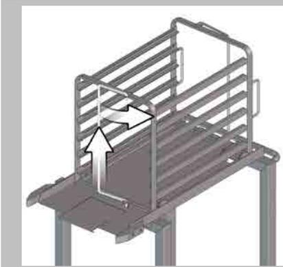
Lift the tray guard bar at the back of the mobile shelf rack and swing it to the right side.
