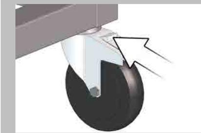
Release the transport trolley's parking brakes.
