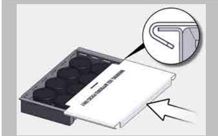
Starting from the back of the box, slide the cover onto the smoker box as far as it will go. Make sure that the folds on the sides of the cover slide along the wings on the sides of the box (as shown in the diagram to the left).
