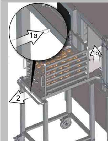
Release the transport trolley's engaging mechanism from the cooking compartment opening and move the trolley away.
