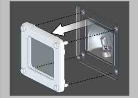
2. Remove the entire assembly from the cooking compartment wall.
