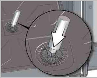
Vertically push the bottle into the pointed tip at the center of the cooking compartment drain so that the tip will pierce the seal.
