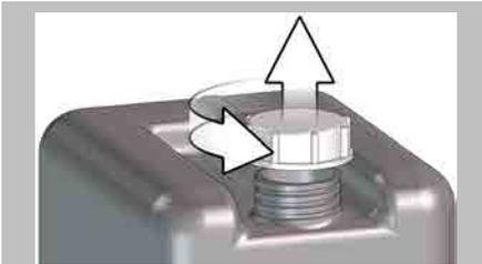
Remove the cap from the ConvoClean new or ConvoClean forte replacement canister.
