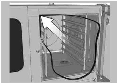
Start by putting the hygienic plug-in gasket back in place at all four corners. Start from one of the upper corners.
