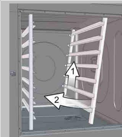
Push(1) the rack upwards and remove (2) it.
