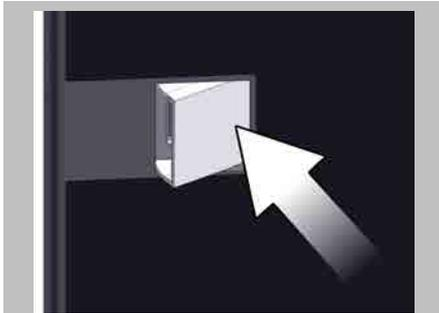
Open the USB port cover on the control panel.
