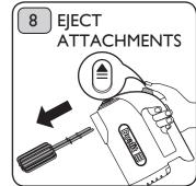
Raise the mixer head and press down on the beater ejector button to eject the beaters. Note: The speed control must be set to '0' to release to beaters.
