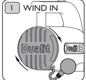
After each use, for easy and tidy storage, wind the power cord into the body of the mixer by turning the swivel base clockwise in the direction shown by the arrow on the mixer body.
