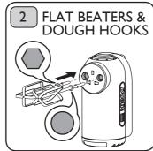
Ensure you insert the correct beater into the correct hole. Match the shape on the underside of the mixer to the shape on the attachment stem. Insert with a slight twist and push action until they click in to place.
