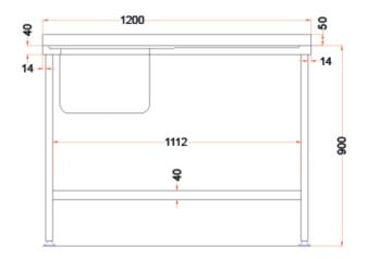
This 1200mm wide flat-packed sink from Holmes features a left side bowl with right side drainer, and is easy to assemble. The sink is made with 304 stainless steel, which is smooth, hygienic and easy to clean whilst offering high resistance to rust and staining making it perfect for use in commercial kitchens. The sink allows you to create practical and hygienic washing areas in your kitchens, and features a strong undershelf for additional storage.
