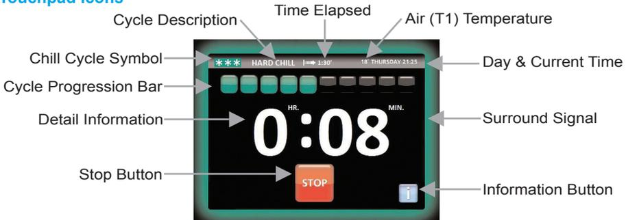
*(Some icons or switches are only visible during adjustment, when activated by parameters or through operation/manual selection).*
