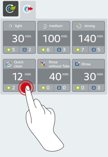
Quick cleaning easily found and quickly activated: simply place the cleaner tabs in the floor drain strainer and start the clean. Production can then resume after no more than 12 minutes.
