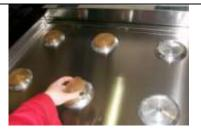
Lift off aluminium burner plates.
