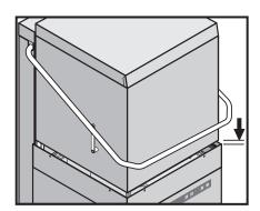
▶ Until the next wash process, place the hood in the stand-by position (engaged position just before closing), to prevent cooling down.
