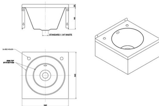
Washbasin top manufactured from 0.9mm thick, grade 1.4301 (304) stainless steel - high polish finish. The apron support is made from 0.9mm (430) material - high polish finish. Prepared for 32mm waste outlet overflow. Supplied with two tapholes in the rear ledge. Wall mounting by using the fixing holes provided in both the rear upstand and the rear apron fixing brackets. Screws and plugs are not supplied.
