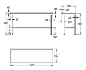
Mini wall tables will align with the Mini range of catering sinks. Mini wall tables are manufactured from 1.2 thick austenitic grade stainless steel polished to a satin finish. Stainless steel underframes complete with shelf are supplied with each table, in a flat pack form with easy to read assembly instructions. Each leg is fitted with an adjustable foot (-20, +10mm) with a working height of 900mm.
