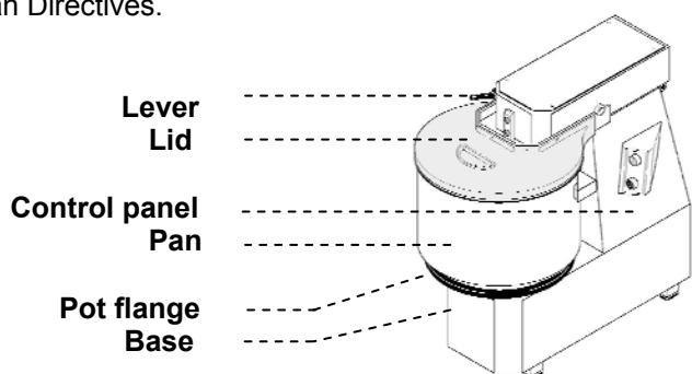
The bowl is removable to allow it to be washed in hot running water or a dishawater.
