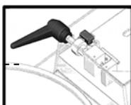
**Sensor:** it prevents the machine from starting if it does not detect the presence of the pot (CNS mod. only)
