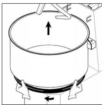
For removing the pan rotate the lower flange clockwise and lift the pan upwards (mod.CNS).
