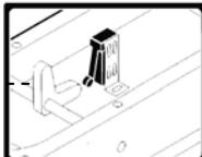
**Remote control switch:** after an unscheduled power cut, it requests a specific machine restart control
