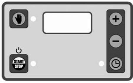
other reason, before lifting the pot's lid, put the machine in standby by pressing the "START/STOP" key again. This will also stop the timer, which will resume together with the machine only by first lowering the lid and then pressing the "START/STOP" button again.
