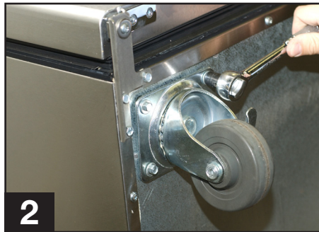
2 Anchor the four screws firmly to the base of the unit.
