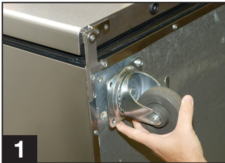
1 Thread four screws into castor in the underside of cabinet frame rail.
