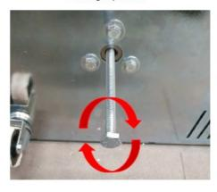
7: When the M10 screw does not screw manually, use the 17 wrench.
