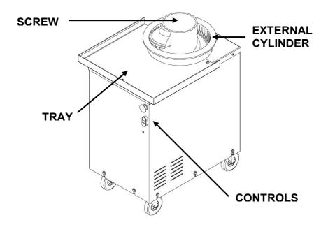
The rounding machine was designed and built **exclusively for use with food**, for the cold processing of wheat based dough in order to round the portions while keeping the fundamental characteristics of the dough unchanged. It is mainly intended for use by pizzerias, bakeries and pastry shops.
