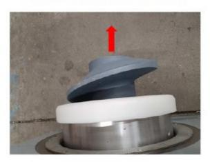
ATTENTION: ONCE THE SCREW IS REMOVED MAKE THE ILLUSTRATIONS PRESENT IN POINT N 6.2 OF THE INSTRUCTION MANUAL PROVIDED: REPASS THE PIN WITH GLASS PAPER UNTIL THIS IS COMPLETELY SMOOTH AND FREE OF SHOTS.
