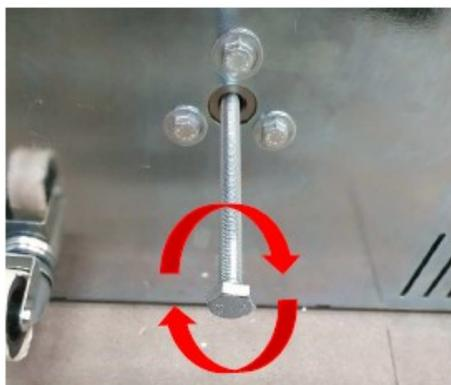
7: When the M10 screw does not screw manually, use the 17 wrench.
