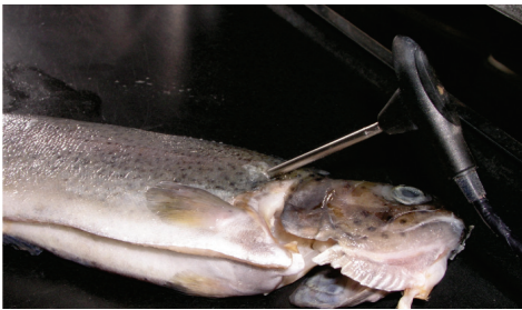
Insert at the thickest point on the fish
