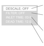
Sets and shows remaining weeks before de-scaling is needed ("DES-CALE TANK" message on the screen). Setting it to OFF will disable the function. Range: 1 – 60 weeks. Default value: OFF
