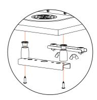
The 2 standard braces can accommodate counter thicknesses up to 40mm. Where the counter thickness is less than 25mm the hard plastic legs on the front brace must be removed and reattached to the other side of the brace using a screwdriver. The rubber inserts in the brace should be removed and repositioned in the plastic legs as shown above.
