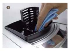
4. Clean hopper Use dry rag clean the channel of hopper. Do not use water to wash hopper channel.
