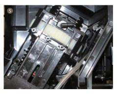
5. Pull the brewing unit outward and rotate the gear clockwise to the position as the picture shows
