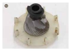
13. Install the screw pin worm drive and conical burr to support lower grindor.
