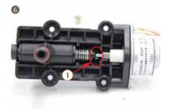
6. Rotate the tail of the stepper motor to make the axis of the stepper motor stand up to the drain valve support until it cannot stand up any more.
