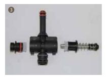
3. Assemble the pin seal, pin and drainage valve pipe into the drainage valve. Pay attention to the direction of the pin seal as the picture shows.
