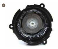
4. Put the already installed epicyclic gear frame A into the gearbox, put 1 filler piece
