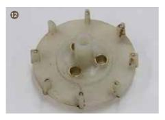
12. Install 3 spring sleeves into the hole of the support lower grinder.
