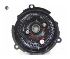
13. Disassemble the 2 screws inside the gearbox, and take out the grinder motor
