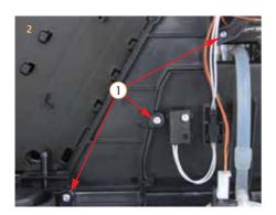
2. Disassemble 3 screws, and take out frame support
