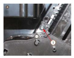
4. Disassemble 3 screws from brew unit
