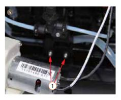
5. Pull out silicon pipe on condensator that connected to pump
