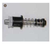
1. Assemble the drain valve support, pin, pin sleeve, pin reset spring, pin seal together as the picture shows. Pay attention to the direction of the pin seal.
