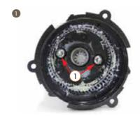
1. Assemble the grinder motor and gearbox together, and screw them tightly. The screw should be covered with loctite. The teeth of the gearbox should be coated with oil(MI-setral-61B). The red mark place should correspond to one hole of the gearbox.
