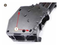
5. Disassemble five hooks at the back of the left and right cover, and take out the left and right cover
