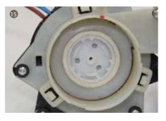
15. Put the felt ring into the already installed coffee powder container.
