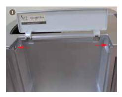
1. Disassemble 2 screws from the left side of the top cover
