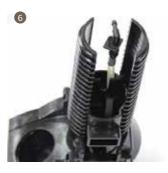
6. Assemble the already installed contropistone into the brew unit frame. Note: The direction of the contropistone should be the same as the picture showed.
