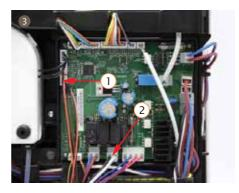
3. Pull out dispenser valve terminal on PCBA, and take it out from the cable rack
