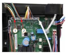
5. Pull out terminal on PCBA which connected to control panel
