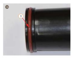
14. Disassemble seal from contropistone
