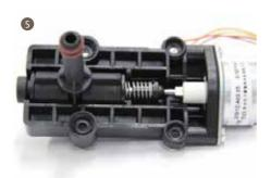
5. Assemble them into drainage valve, and install the seal, Teflon pipe and clamps.
