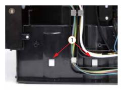
8. Disassemble hooks from the support and take out thermoblock
