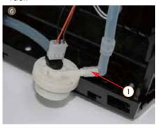
**6.** Pull out the flowmeter and pull out the silicone pip
