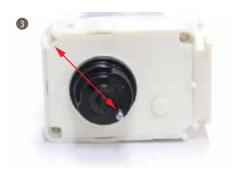
3. Install the gear box lid and sheave drive part, pay attention to the position of the sheave drive part.
