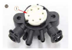
12. Assemble the ceramic plate C on dispenser valve silicon plate, the smooth side should be covered with oil(SYN-setral-AI/C 2-FD).
