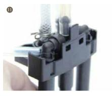
11. Pull out all the silicon pipes
