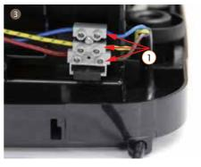
3. Disassemble 1 screw from support, loose 3 screws inside the line pencil connector and take out the power cord
