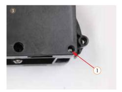
3. Disassemble the 4 screws from the left and right cover
