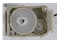
2. Install dispenser valve gear A and dispenser valve gear B into dispenser valve gearbox after coat oil(MI-setral-61B).
