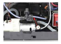
3. Pull out Teflon pipe on dispenser valve 2W that connected to pump, and take out dispenser valve 2W
