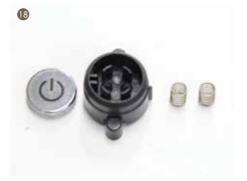
18. Take out the spring and the power button, and disassemble power button decorative cover
