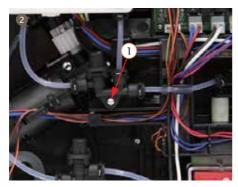
2. Disassemble 1 screw from dispenser valve 3W so that the wiring cable can be taken out from the cable rack.
