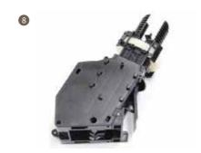
8. Install the left and right pull plate and left and right cover on brew unit frame, oil (MI-setral-61B) coating position for left and right pull plate should be as the picture shows.
