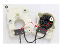
5. Install microswitch line pencil switches to sheave permanent seat and dispenser valve separately. Pay attention to the position and the direction of the sheave and microswitch.
