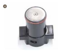
4. Coating the contropistone seal with lubricating oil(SYN-setral-AI/C 2-FD) and install to the contropistone, and then lock the filter screen.
