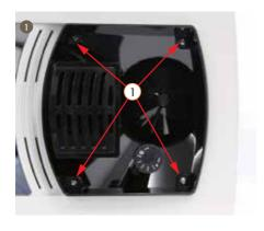
1. Disassemble 4 screws from the coffee bean container, and take the coffee bean container out
