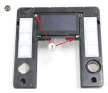
23. Disassemble 2 screws from display screen, and take out the OLED screen
