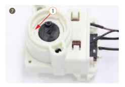
7. Install the ceramic plate A into the dispenser valve. The upper side should be the side of slot, and it should be covered with oil(SYN-setral-AI/C 2-FD).
