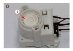
8. Install the ceramic plate B into the dispenser valve. Both sides should be covered with oil((SYN-setral-AI/C 2-FD).
