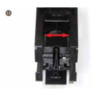
11. Deform brew unit frame with strength according to the arrow direction, and take out coffee brewing group
