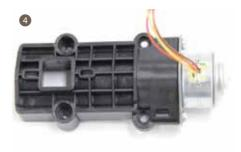
4. Put the stepper motor and drainage valve support lock together. Pay attention to the direction of the stepper motor.
