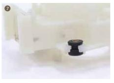
7. Install 3 grinder antivibration pads and 3 antivibration bushes into coffee powder container.
