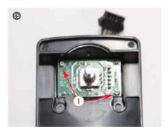
15. Disassemble 2 screws from the rotary, and take out the bottom terminal, and then take out the rotary PCB
