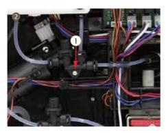
2. Disassemble 1 screw from dispenser valve 3W so that the wire can be taken out from the cable rack
