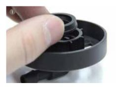
1. When installing the support seal, the downside should be with bigger diameter.
