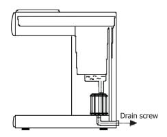
Re-tighten the water drain screw firmly afterwards.
