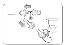
1. Assemble the hose connector (A), and attach it to the end of the accessory hose as shown.
