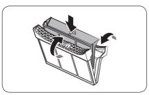
5. Put the inner filter into the outer filter, and then reinsert the lint filter into the original position.
