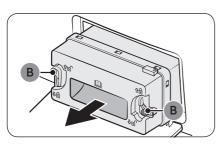
2. Unlock the inner cover fixers (B), and then pull the inner cover to remove.
