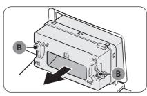
2. Unlock the inner cover fixers (B), and then pull the inner cover to remove.
