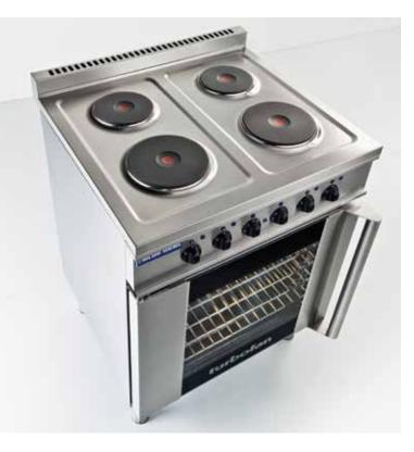
The new and improved E931M light commercial range takes 4 gastronorm GN 1/1 Pan capacity with 80mm spacing. The 4 element cooktop offers two 2kW high speed front elements and two 1.5kW high speed rear elements all contained with the new full hygienic pressed stainless steel top. The convection oven is a versatile oven that can roast , grill, bake and is ideal for use in compact applications that require an oven / cooktop that is versatile.
