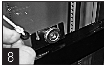
Door roller bracket with nylon cord.
