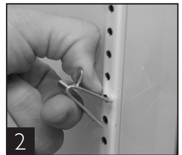
2 Installing bottom of the shelf clip
