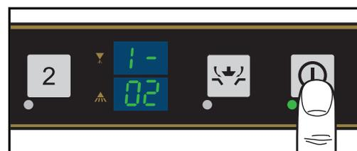
↳ When the value changes, the LED of the ON/Escape key illuminates for 3 sec.
