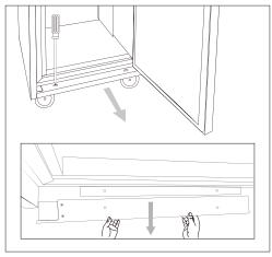
Remove the right top hinge and bottom hinge to release the door. Then remove the door carefully.
