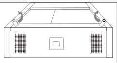
2. Lift the controller panel upward for about 15mm, then take it out.
