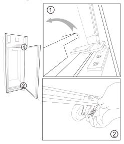
6. Mount the left top hinge and bottom hinge with screws. Keep the top hinge a little loose so that the door can be inserted later easily.
