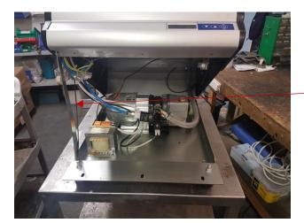
**Step 4:** Lift the super structure completely, taking care not to pull the electrical plant. Use a metal rod located on the left hand side, inside of the machine, to secure the superstructure in an "Opened" position.
