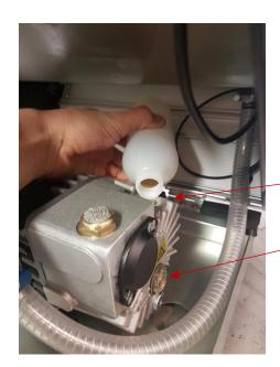
**Step 8:** Pour new oil into the oil loading hole making sure you do not go above the "Max" Line located on the side of the "Oil inspection window".
