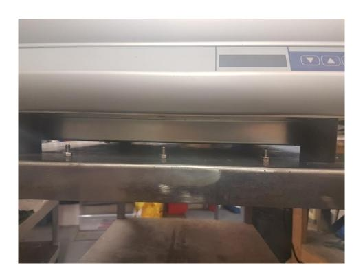
**Step10:** Lower the super structure (making sure no electrical components have been disconnected during the oil change procedure) and fasten the three profile locking screws.
