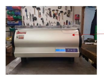
**Step 2:** Place the machine on a worktop high enough to allow a basin to be placed underneath to collect oil and make sure the chamber lid is in a closed position.
