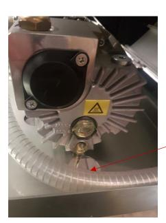
**Step 6:** Allow the used oil to drain into the basin underneath. Once the pump chamber is emptied completely, screw the oil drainage plug back in place.
