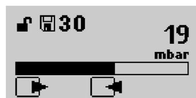
Fig. 33: Gas flushing status display (049)
