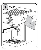
Remove the Grouphead Heat Shield and use a damp cloth to clean the Steam Wand. Grouphead, Grouphead Heat Shield and Showerhead. There should be no milk residue or coffee grounds visible. Then reinstall the Grouphead Heat Shield.
