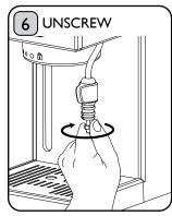
Unscrew Steam Nozzle in a clockwise direction (when viewed from above) to remove from the Steam Wand. Do not apply excessive force. \*
