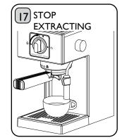
Once desired volume of coffee has been extracted. turn the Function Selector Knob to 'Off' position. A I Cup Filter Basket should take 20-30 seconds to extract, a 2 Cup Filter Basket should take 25-35 seconds to extract.
