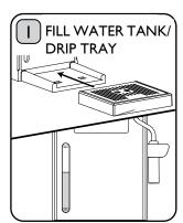
Ensure that the water level is above MIN and below MAX. DO NOT USE ANY OTHER LIQUID. **Do not overfill.** Ensure that the Drip Tray is empty and in position.
