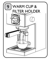
Water will dispense into cup, warming the cups, Cup Filter and Filter Holder for a hotter drink and ensuring they are clean and not blocked. When desired volume of water has been dispensed, turn Function Selector Knob to 'Off' and place cup to one side.
