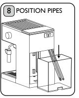
Position Water Tank Pipes in Water Tank.
