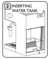
See page 11 to ensure the protective bag has been removed from the Water Tank Pipes. When inserting Water Tank, lift **both** pipes up and place down into the Water Tank, before insertion. The Water Tank Pipes must hang down into the water as shown, when Water Tank is fully inserted. If the Water Tank Pipes are not as shown, remove Water Tank, pull Water Tank Pipes down and insert again.
