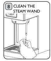
Use a pin to remove dried milk from inside the Steam Wand.
