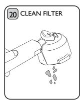
Remove Filter Holder from out the grounds over a bin. water to remove any coffee grounds. Use a pin to unblock if required. Caution: Filter Holder will be hot. Always hold by the handle, do not touch the metal Filter Basket. Risk of burns and
