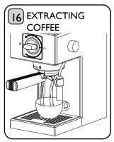
Empty dispensed hot water from cups and place under the Filter Holder ensure cups are directly under both nozzles. Turn Function Selector Knob to Coffee/Hot Water Function. You will hear the pump operating. Flow for an espresso will begin 5-8 seconds after function selection.
