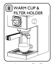
Insert the empty Cup Filter and Filter Holder into the Grouphead. Place cup under Grouphead and tum Function Selector Knob to Coffee/Hot Water Function. Ensure that the Steam Wand is positioned over the Drip Tray when not in use.
