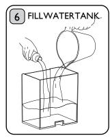
Fill the Water Tank with recommended amount of descaler (see instructions of your descaler) and fill to MAX line with water. Then reinstall the water tank. DESCALE AT LEAST ONCE A MONTH IN HARD WATER AREAS.
