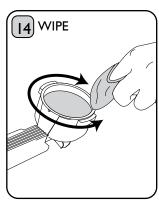
Wipe the rim of the Cup Filter to remove excess ground coffee. If you don't, a watertight seal will not form and water or coffee will leak from the Brewhead.
