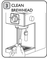
Use a pin to clear holes and grooves, and clean with a soft brush. Dry, then use a screwdriver to reinstall the Showerhead.
