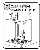
Support the Steam Wand then pull the Steam Wand Handle down to remove. Note: Steam Wand Handle is tightly fitted and may need extra time and attention to remove. Clean Steam Wand Handle with detergent and a cleaning brush.
