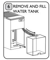
Remove the Water Tank from the back of the appliance and remove the protective bag over the Water Tank Pipes. Rinse before filling with fresh water. DO NOT USE ANY OTHER LIQUID.
