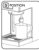
Without the Filter Holder in place, place the Steam Wand into a deep lug.
