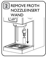
Pull the Froth Nozzle downwards to remove. Position the Steam Wand into a deep lug or Teapot.
