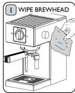
Wipe the entire Brewhead area and external surfaces to ensure it is completely free of coffee grounds. Fine coffee grounds can block the Shower Head.
