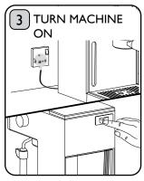
Plug the Power Cord into the mains supply and press the Power Switch into the 'On' position.
