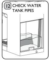
When inserting Water Tank, lift **both** Water Tank Pipes up, and place down into the tank, before insertion. The pipes must hang down into the water, as shown, when Water Tank is fully inserted. If the Water Tank Pipes are not as shown, remove Water Tank, pull Water Tank Pipes down and insert again.
