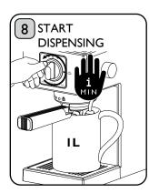
Turn the Function Selector Knob to the Coffee/Hot Water Function to start. Allow the descale solution to dispense for I minute. Do not engage the Steam Function. **Risk of chemical inhalation.**
