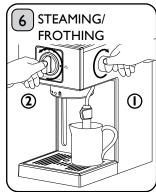
**Step I:** Once milk reaches desired amount of froth. turn Steam Flow Control Knob clockwise.
