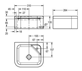
Drinking water fountains are manufactured from grade austenitic stainless steel, material thickness 1.2mm, supplied complete with 19mm waste and water bubbler. The wall mounted model is simply fixed to the wall using a joggle strip and integral mounting brackets.
