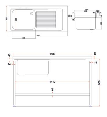
The 1500mm wide flat-packed sink from Holmes is a made with industrial grade 304 stainless steel, which offers high resistance to rusting, stains and makes it easy to clean. The sink is designed with a left side bowl and right side drainer, and is easy to assemble. Create practical and hygienic designated washing areas in your kitchen with this reliable commercial sink, which also benefits from a sturdy undershelf offering support for heavy appliances or extra storage.
