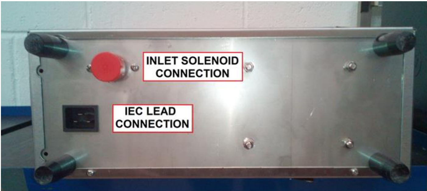
Figure 8 - Base of SP9 Undercounter Unit
