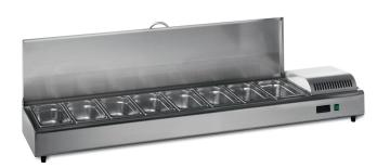
Prepare perfect pizzas and sandwiches either at the front of house or back of house with the Seal Food Display Bar. Holding food at 3°C-7°C in ambient conditions up to 25°C, its low profile enables it to hold 100 mm gastronorm containers.
