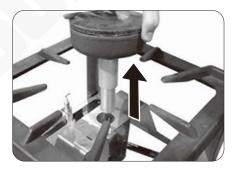
3. Unscrew the 1.15mm injector and save for future use.
