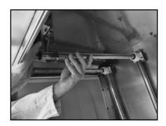
► Lower: Lift the rinse arm and pull it out to the front.
