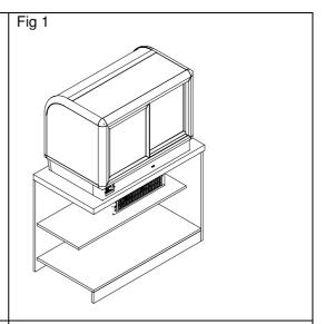
The dimension X from the front grille of the condenser to the inner face of the counter front must not be less than 200mm.
