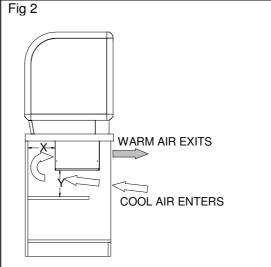
If it is required that the rear of the counter is enclosed using doors or a fixed panel, then adequate vents must be provided to allow air to pass through these fixtures.
