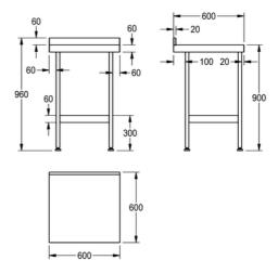
Mini wall tables will align with the Mini range of catering sinks. Mini wall tables are manufactured from 1.2 thick austenitic grade stainless steel polished to a satin finish. Stainless steel underframes complete with shelf are supplied with each table, in a flat pack form with easy to read assembly instructions. Each leg is fitted with an adjustable foot (-20, +10mm) with a working height of 900mm.
